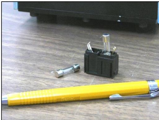
FUSES ARE RATED FOR 250V / 5A AC
