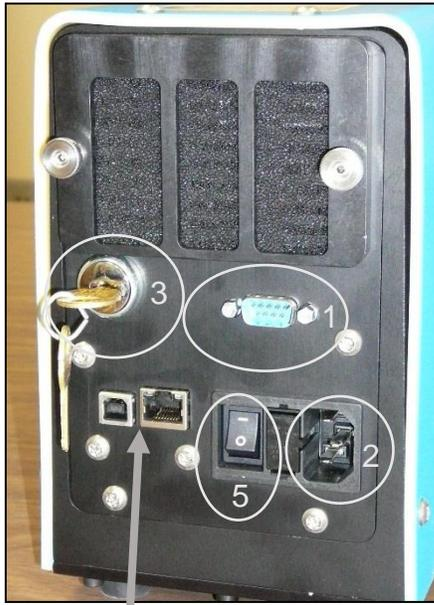
1. Attach the included RS-232 cable from the LABELASE® 1000P Plate printer to your Windows-based PC running LabeLase® Producer™ software.
