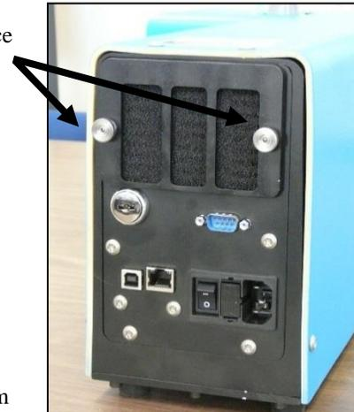
Loosen the thumb screws and carefully remove the cover and the foam filter element underneath.
