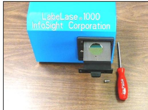
**CAUTION: DO NOT TOUCH LENS WITH FINGERS OR ANY SUBSTANCE CONTAINING ALCOHOL, OR PERMANENT DAMAGE MAY RESULT.**
